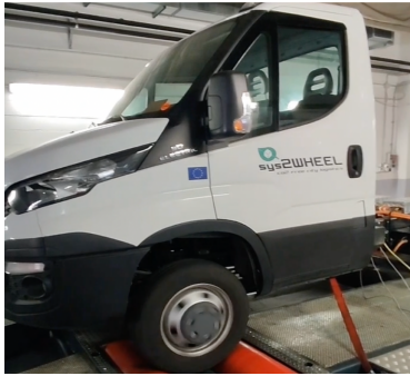
Figure 2: N2 Category vehicle IVECO Daily with fully modular e-axle on roller test bench for evaluation ( source )
