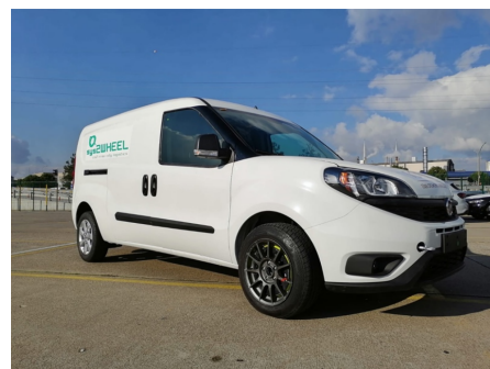
Figure 1: N1 category vehicle on the test track: Fiat Doblo with in-wheel technology and increased space for cargo or battery in the rear by close-to-wheel suspension ( source )
