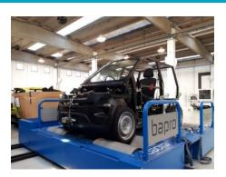
Figure 9: Energy efficency testing of the TELL vehicle on the rolling road at I-FEVS
