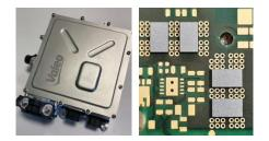
Figure 7: VALEO inverter including: (left) Power circuit based on Si Mosfets and (right) Power circuit based on GaN transistors
